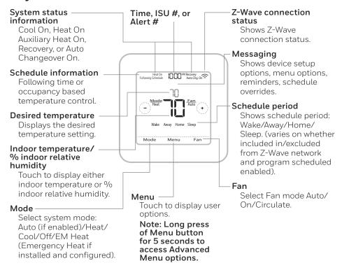
The screen will wake up by pressing the center area of the displayed temperature. If powered by 24 VAC, the screen stays lit for 45 seconds after you complete changes.
